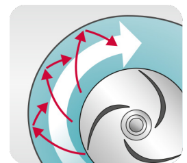
Flygt impeller keeps solids moving with the flow.
